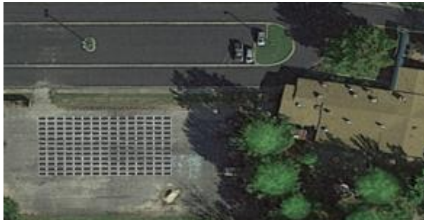
Figure 2.7: Aerial View of Concept Plan for Clubhouse Site Using Same Low-Profile Ballasted Ground Mount (GRM) Rack Solution
